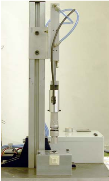
Fig. 5: Test facility for mating durability
