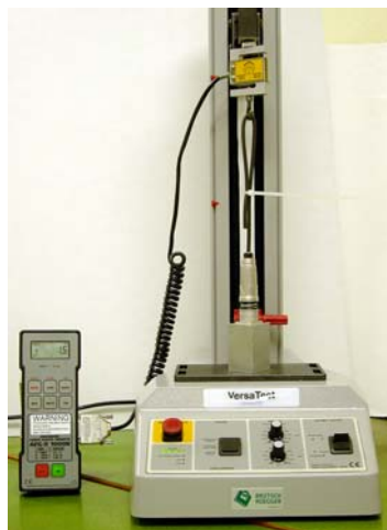
Fig. 3: Equipment for examination of cable retention
