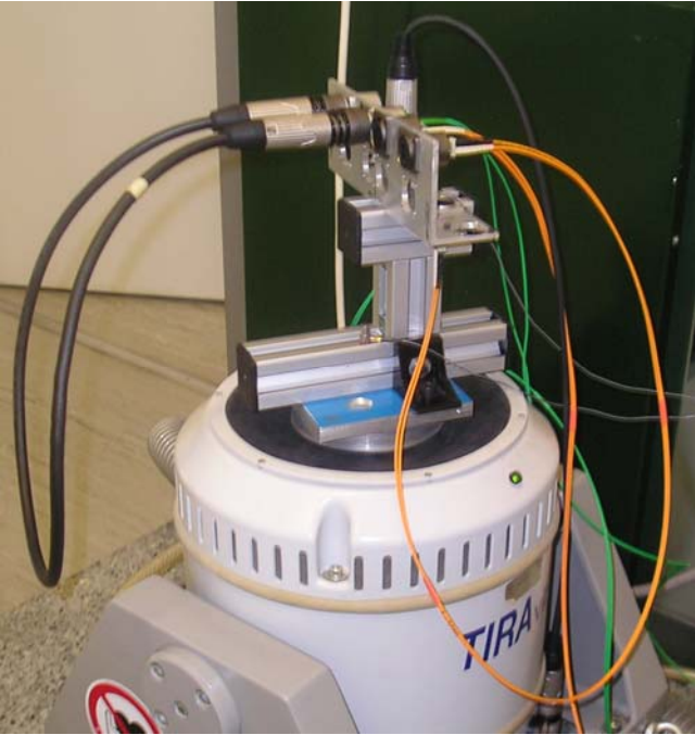
Fig. 2a: Vibration equipment and test cable arrangement
