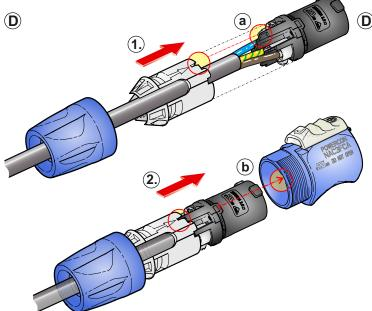
D Slide the insert and the chuck (1) into the housing (2).
