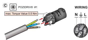
© Insert the wire into the terminals and fasten the clamping device with a POZIDRIV® #1, max. Torque 0.5 Nm (0.37 lb-ft).
